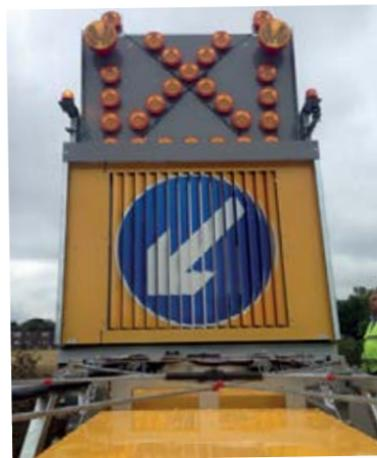
displayed, regardless of conditions. If the power to an LED VMS is cut, no message will be displayed. On a prismatic VMS, the same message as before the power cut will be shown. Furthermore, as the Triplesign prismatic can also be manually operated with a 6mm Allen key, it is still a variable message sign even if there is no power.
